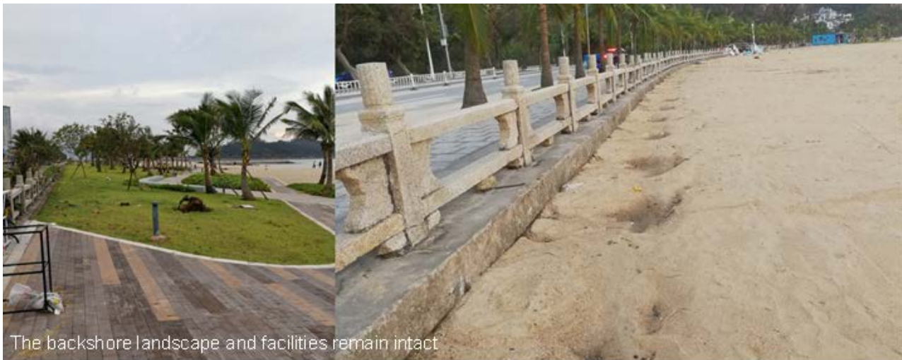
Figure 19. The coastal guardrail and backshore facilities protected by the restored beach remained intact during the super typhoon (Source: Third Institute of Oceanography, Ministry of Natural Resources)
