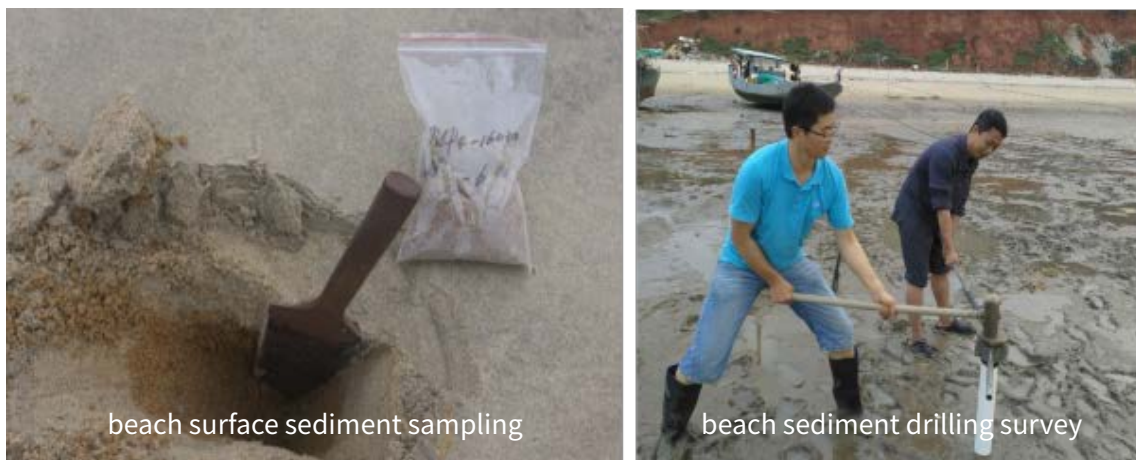
Figure 2. Collection of Surface Sediments and Core Samples from Beaches (Source: Third Institute of Oceanography, Ministry of Natural Resources)
