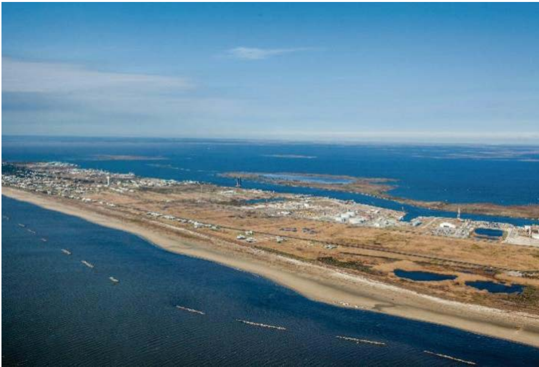
Fig.33 Oyster Reef Ecosystem Restoration for Marine Hazard Mitigation along the Coast of Louisiana, USA, using a similar breakwater design as in Alabama, photo credit: Erika Nortemann/TNC.
