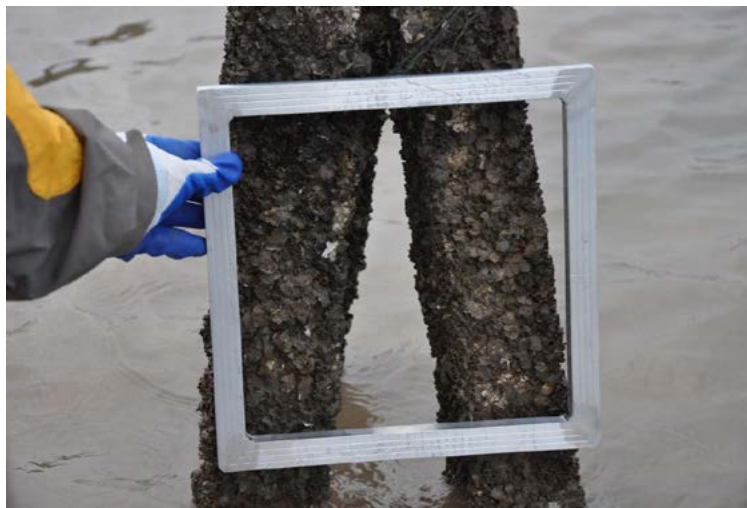
Fig.28 Monitoring of the Settlement Effect of Artificial Reef Structures
