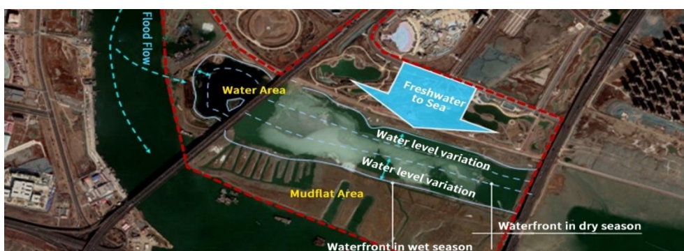
Figure 12 Schematic Diagram of Water System Connectivity outside the Seawalls.
