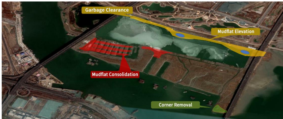
Figure 3 Distribution Map of Engineering Measures in Wetland Remediation Area outside the Seawalls.
